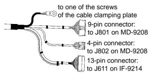
Figure 5-7 Signal cable, antenna unit side
